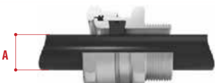
Cable gland with gasket with unarmoured cable
